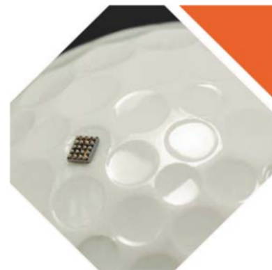
Figure 2: The NXP Kinetis KL03 20-pin ARM® Cortex®-M0 powered MCU, at 1.6 mm x 2.0 mm, is suitable for ingestible healthcare sensing. The KL03 (MKL03Z32xxx4) supports 32 KB Flash, 2 KB SRAM, 8 KB boot ROM, and up to 22 GPIO.
